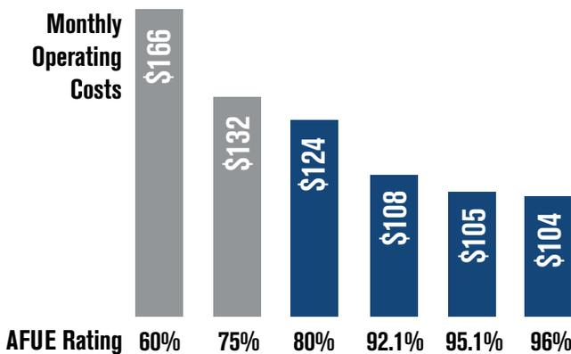
Dollar amounts computed at \$.092 ccf, for 2,500 full-load heating hours and a system rated at 60,000 Btuh. Actual costs vary depending on climate conditions, fuel rates, and patterns of usage according to individual lifestyle.
