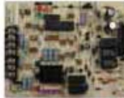
All Maytag M120 gas furnaces feature a state-of-the-art SmartStart® control board that learns the start-up characteristics of the furnace as installed in your home. It adapts to the most efficient start-up time, extending the life of the igniter.
